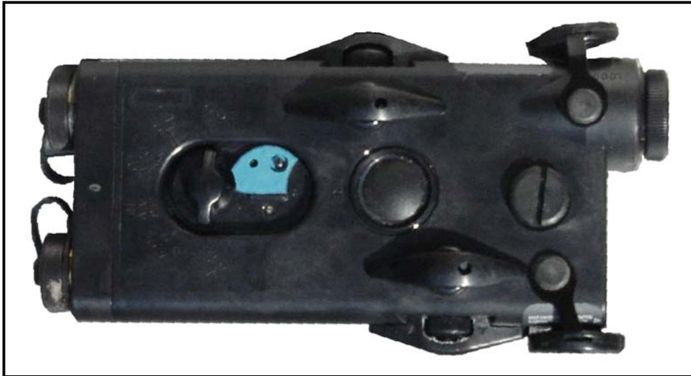
Figure 2-30. AN/PEQ-2A target pointer illuminator/aiming light.
