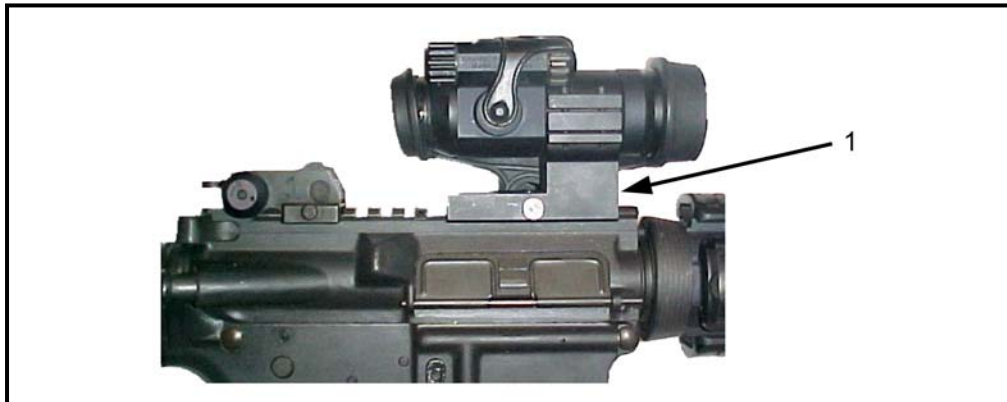
Figure 2-25. M68 mounted on the M16A4/M4-series weapons.
