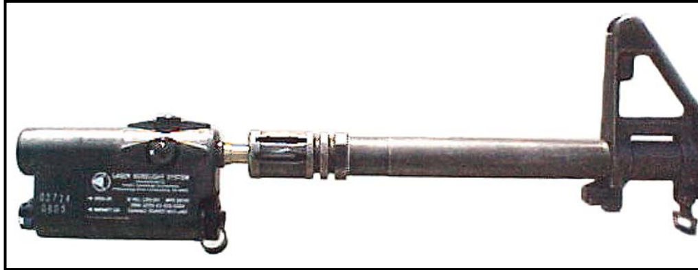
Figure 8-4. Borelight in the HALF TURN position.
