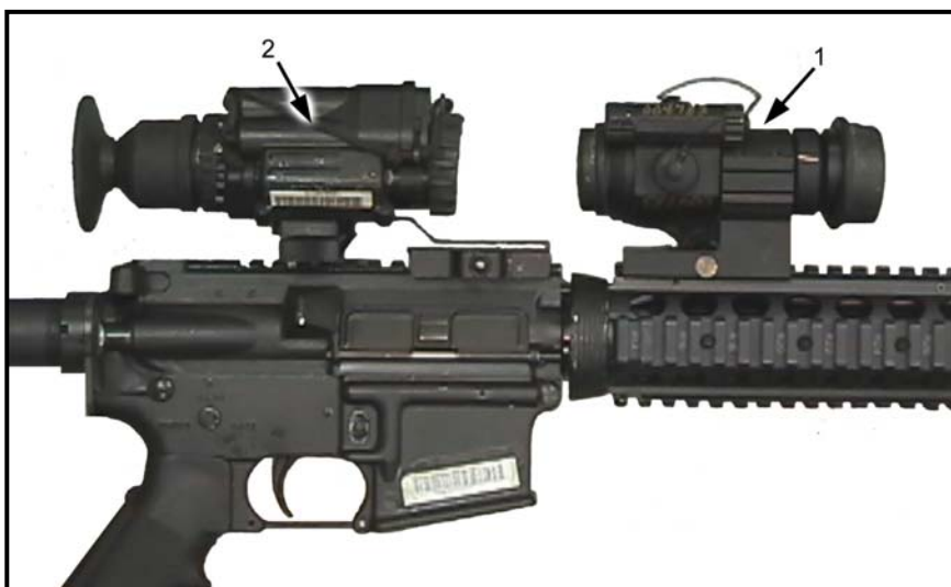
Figure 2-26. Mounting the M68/AN/PVS-14 combination on an MWS.
